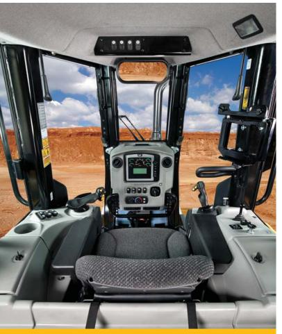
An isolation-mounted pressurized cab reduces dust entry, noise and vibration. Large glass panels provide excellent visibility. Intermittent wipers maximize visibility in poor weather conditions. Heating and air conditioning controls are conveniently located. Temperature control is automatic.
