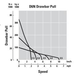
The direct injection electronic fuel system provides a controlled fuel delivery increase as the engine lugs back from rated speed. This results in increased horsepower. A combination of increased torque rise and maximum horsepower improves response, provides greater drawbar pull and faster dozing cycles.
