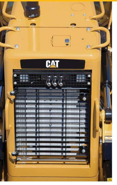
The engine radiator, Air To Air After Cooler (ATAAC), and hydraulic oil cooler are packaged in a single plane. Aluminum bar plate construction provides durability and allows for higher heat transfer and superior corrosion resistance. The standard cores feature 8.9 fins per inch (6.5 fins per inch for the Waste Handling Arrangement) to allow debris to pass through and reduce plugging.
