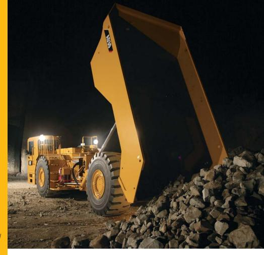
The AD30 underground articulated truck is designed for high production, low cost-per-ton hauling in smaller underground mining applications. Rugged construction and easy maintenance guarantee long life with low operating costs.
