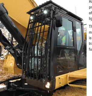
Halogen lights provide plenty of illumination. Cab and boom lights can be programmed to stay on for up to 90 seconds after the engine has been turned off to help you safely exit the machine. Optional High Intensity Discharge (HID) lights are available for enhanced night-time visibility.
